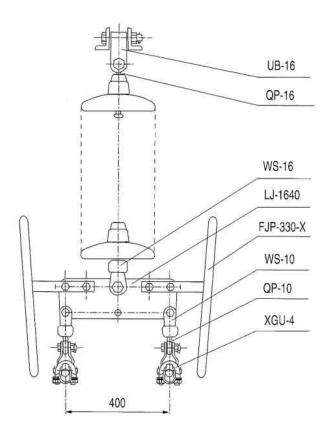
Single Suspension String for Four-Bundle Conductor(Using Yoke Plate with Type LK)
